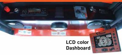
The controls in the cabin are very ergonomic and all monitoring views are displayed on a LCD dashboard monitor. The display is simple and optimized to give you all the necessary informations for effective operations. Moreover, if an alarm occurs, you will not have an incomprehensible code, but a full description of the problem in the LCD display.
